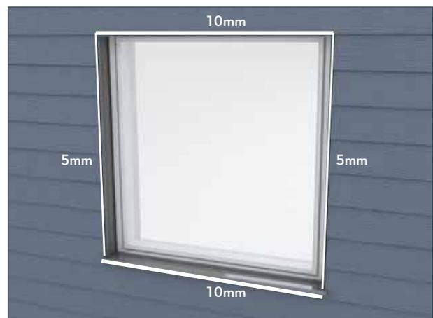
If using untreated timber battens, we recommend using Cembrit EPDM 45/95mm to keep water out.
